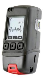
This stand-alone data logger measures and stores over 250,000 temperature readings over a -30 to +80°C (-22 to +176°F) range at a resolution of 0.1°C
