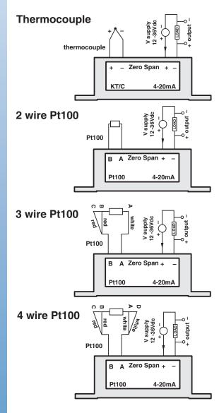
**Note 1:** The transmitter can be easily ranged and calibrated by means of the multi-turn zero and span adjusters in conjunction with either a mV source or standard resistance input.
