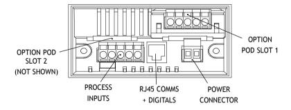
The diagram below shows the rear panel positions for all electrical connections.
