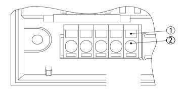
To make a connection: Insert small screwdriver blade into tension clamp orifice (1), push and twist to deflect clamp into open position. Do not lever screwdriver thus forcing connector body sideways. Insert conductor tail sufficiently into (2) then release screwdriver. Ensure no loose wire strands protrude.
