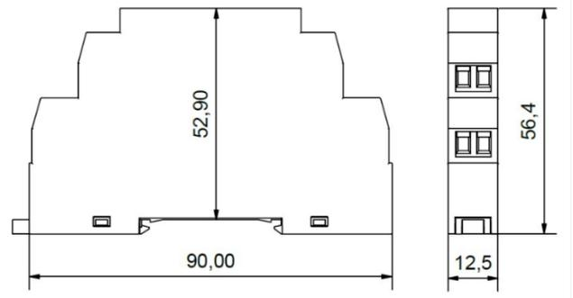
The equipment must be mounted on a DIN rail style DIN EN50022 inside a plastic or metal enclosure with a protection level  $\geq$  IP65. All wiring must be secured. Maximum cable sizes 2.5 mm<sup>2</sup>. Connection clamp terminals.
