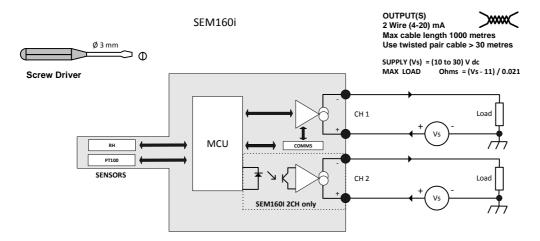
Note:160i/HP/2 channel version: Power must be applied on CH1 for Ch2 to operate correctly
