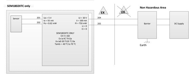
Sensor wires must be isolated from earth breakdown voltage 500 V dc
