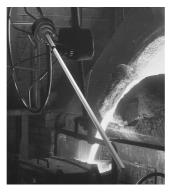
Fig 25: Rare Metal Thermocouple
