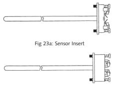
Fig 23b: Sensor Insert with Fitted Transmitter
